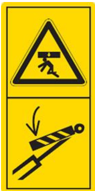
Work on the machine is only permitted when the cylinder protective device is in place
