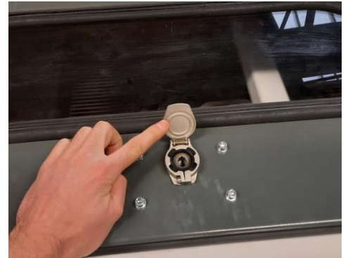
Figure 8. Roof hatch lock
