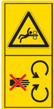
Danger due to rotating parts
