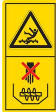
Never reach into or step into the container when the machine is operational
