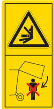
Do not stand under the cutting flap until the shield is in place
