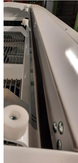
Figure 17. Roof hatch sealing
