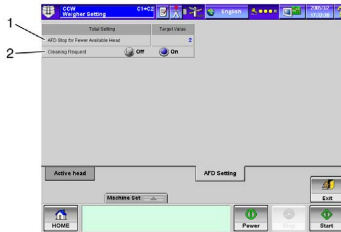
Fig.6-170 [AFD Setting] Tab Screen ([Weigher Setting] Screen)
