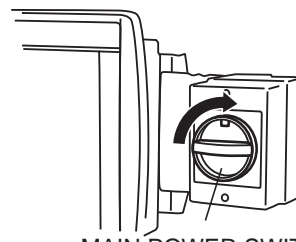
MAIN POWER SWITCH
