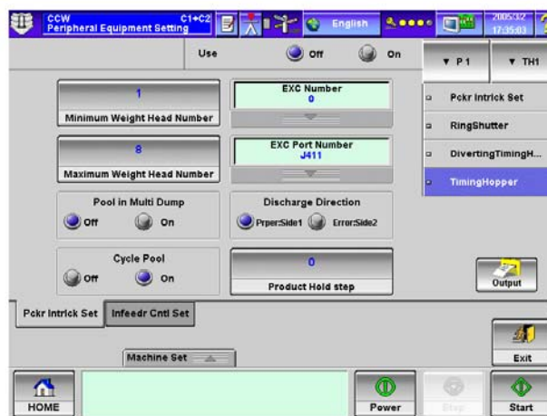
Fig.6-175 [TimingHopper] Index Screen ([Peripheral Equipment Setting] Screen)
